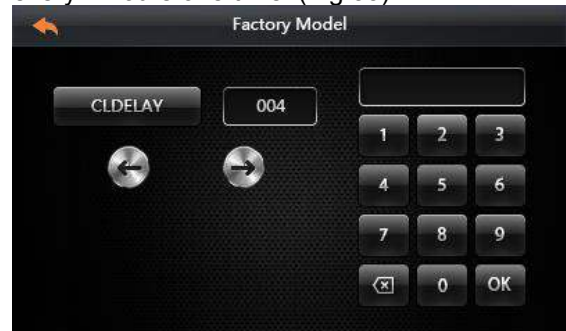
Fig.53 21·Setting the time delay of feeding after successful ignition, for example: start to feeding the pellet in 120s
